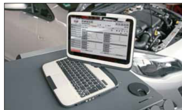
Rotatable monitor for use as a touch screen or with keyboard
